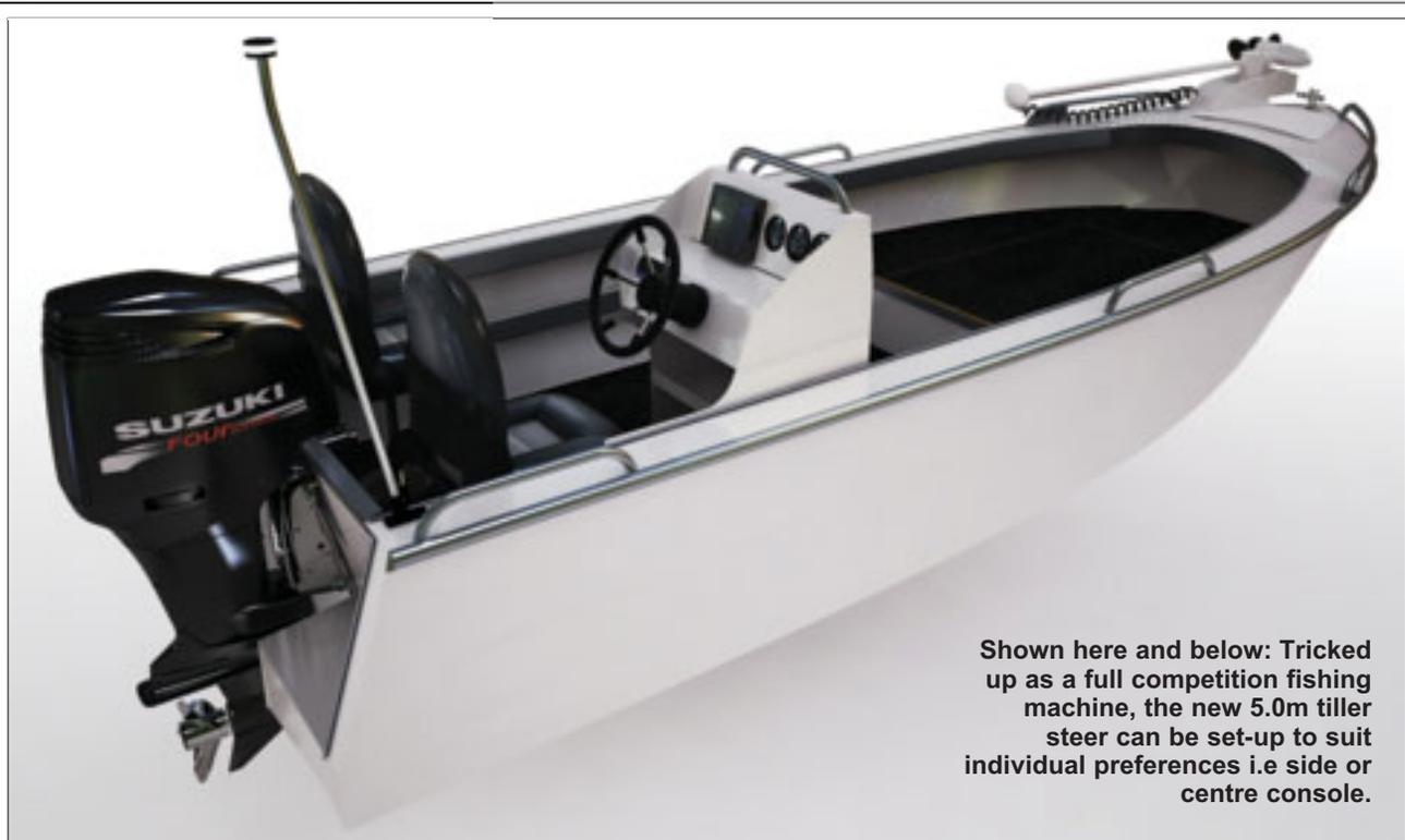
Shown here and below: Tricked up as a full competition fishing machine, the new 5.0m tiller steer can be set-up to suit individual preferences i.e side or centre console.
