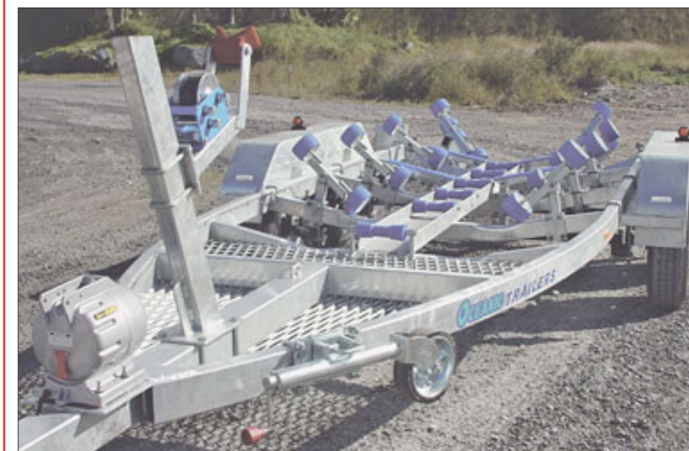
Above: How simple, how much easier it is to hitch up the boat if you can just walk down the walkway provided. Note paired rollers holding the stem in position. Because of the keel extrusion all tinnies use - the boat must come up between the pair of rollers.
