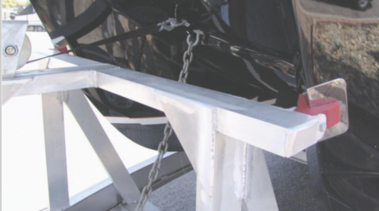
**In either plate, pressed ally or fibreglass, the idea of using wear pads on the boat's stem(s) has real merit, and can save a lot of paint and scoring down the track. Even though the boat is back-chained to the winch post - the post itself still moves as the trailer flexes underneath it.**
