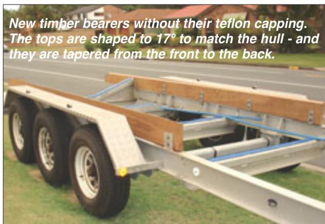
*New timber bearers without their teflon capping. The tops are shaped to 17° to match the hull - and they are tapered from the front to the back.*
