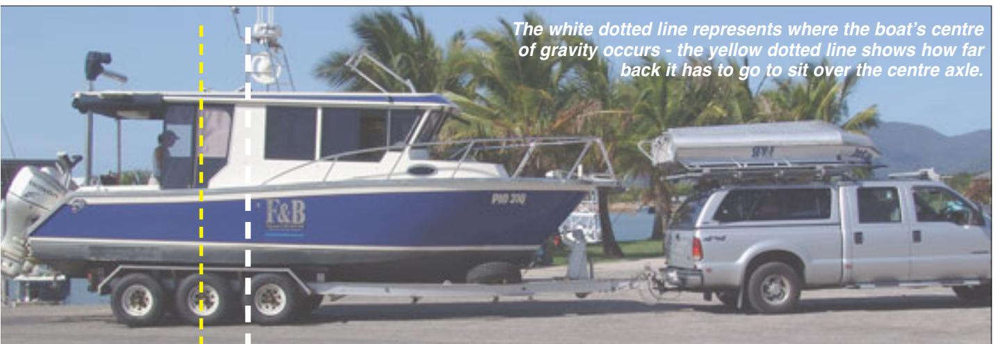
The white dotted line represents where the boat's centre of gravity occurs - the yellow dotted line shows how far back it has to go to sit over the centre axle.
