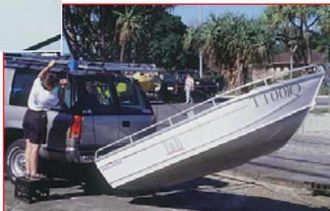
Left: There's nothing to do after the ropes are hooked on, apart from checking the ropes are all clear and ready . . . Above: For you to start winding the winch. There's not a lot of pressure here; even an old bloke or women could wind it - and there's a press button power winch option if they can't.
