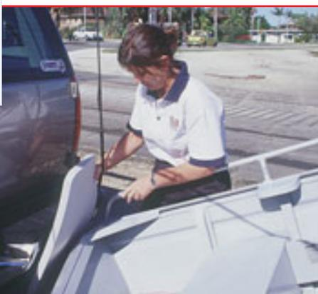
It pays to have a fender handy when the 'weight' of the boat comes on. As the boat lifts off the ground, it comes back hard against the vehicle, as the ropes are literally levering the dinghy up against the vehicle.
