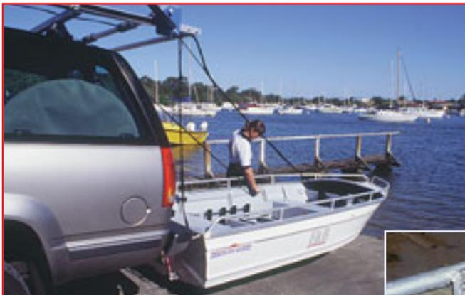
It only takes a few seconds to connect the four snap hooks from the four lengths of polly rope; Rhino added 2 eyebolts (inset) amidships, but just used the Horizon's grab handles on the stern for the aft snap hooks.
