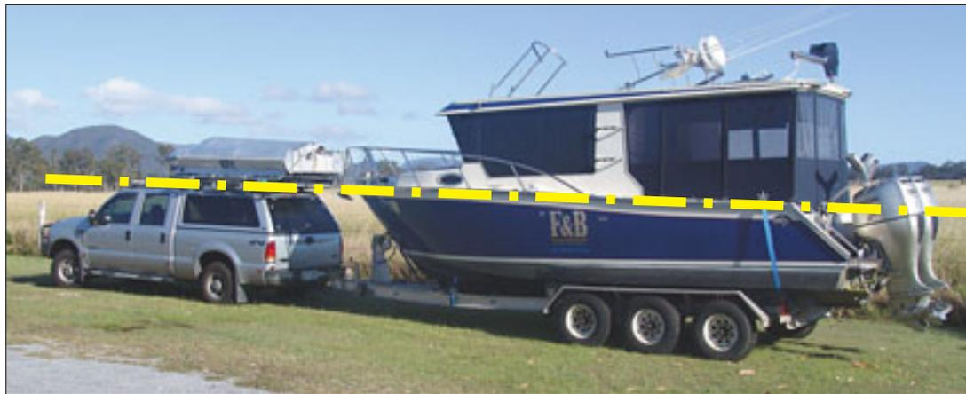
**Same tow vehicle, same trailer, different boats. Given *Far-Away* is a seriously big trailerboat that even makes an F-250 look small (!) check how high the Honda powerheads are relative to the overall height of the Ford. They are nearly 2 metres off the ground. This was our worst point - a horrible set-up. Check the bent chassis going forward; the down angle on front axle - awful, and yes, we blew-out 3 of the 4 front tyres. We got it right in the end, but wouldn’t do it again.**
