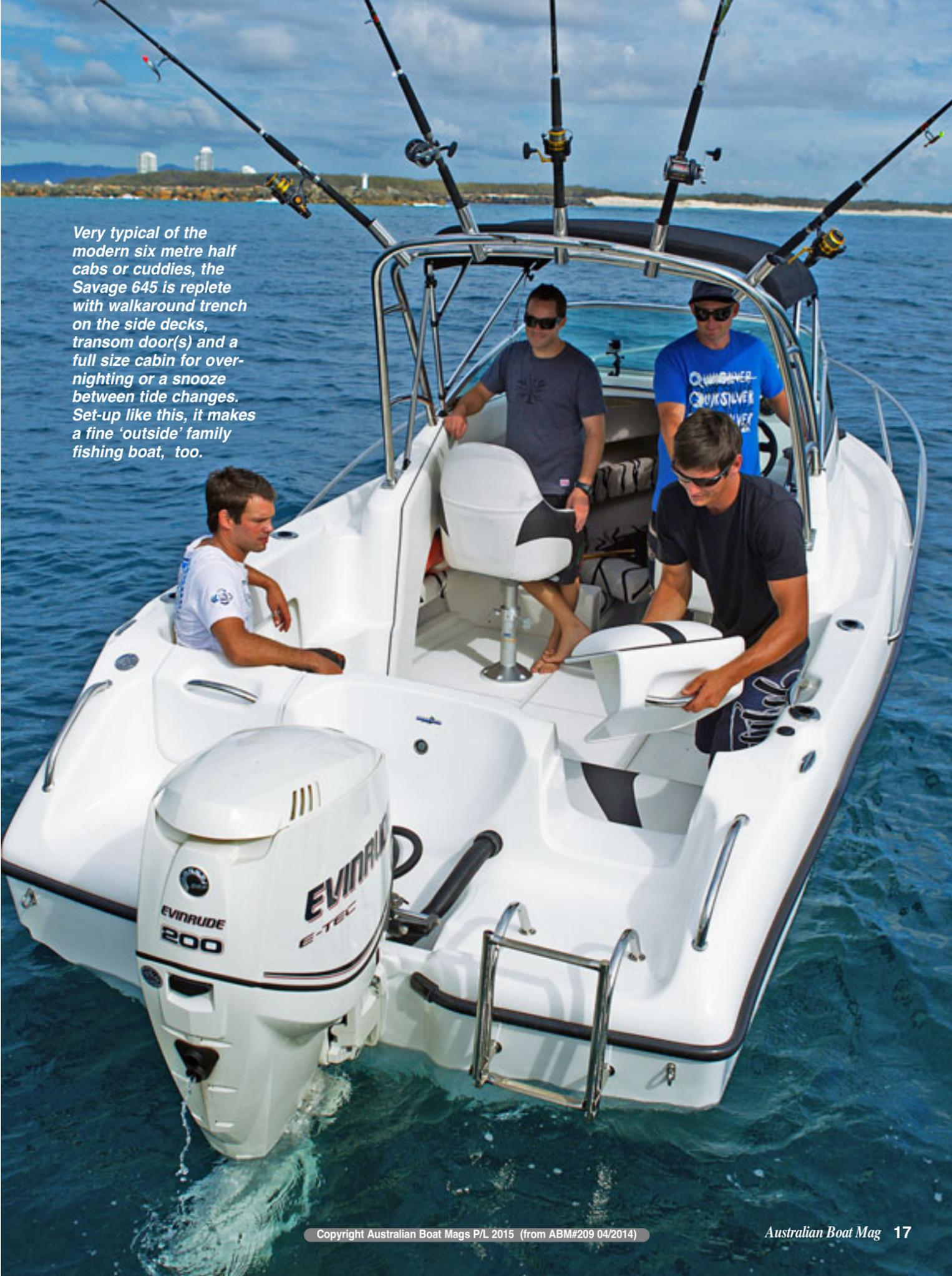
Very typical of the modern six metre half cabs or cuddies, the Savage 645 is replete with walkaround trench on the side decks, transom door(s) and a full size cabin for over-nighting or a snooze between tide changes. Set-up like this, it makes a fine 'outside' family fishing boat, too.
