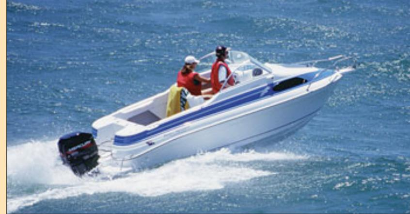
Heading out, Greg Haines carefully steers the boat about 10 degrees of top dead centre, presenting the boat at a slight angle to the waves. Going in head-on is pretty hard on the crew and the boat; bear away 10 degrees or so, and the ride becomes infinitely more comfortable.
