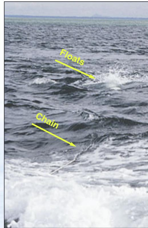
**Top Right:** Way to go - the anchor lifted right up to the surface using the boat's power, not your back.
