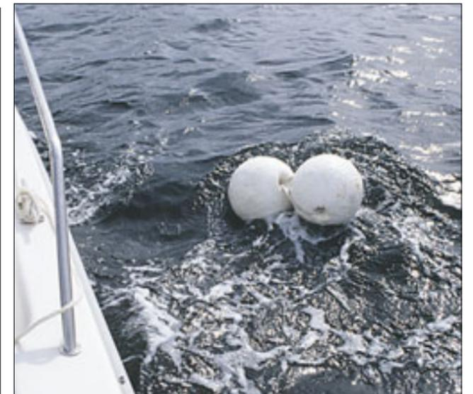
**Bigger boats require bigger anchors, and often, two floats are needed to lift them - especially if the anchor stock has been filled with lead to create a lower scope angle for better holding power.**
