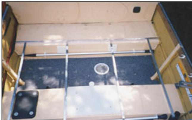
Plastic rocket tubes stop the seats at the rear from lifting and the seat backs sitting against the rear bulkhead stop them from falling backward when sitting in the seats. The whole thing lifts out to make way for the fly-casting platform.
