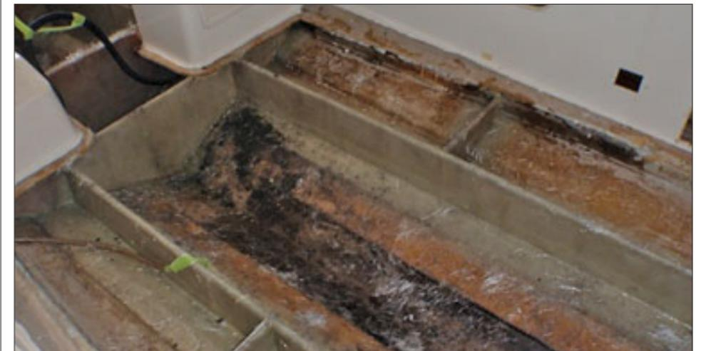
the tank so we couldn't lift the height. The bottom of this tank was also a typical V shape due to the hull. And this is where we found that the V angle was the same from front to back, whereas the hull deadrise angle changed in this length. This would possibly
