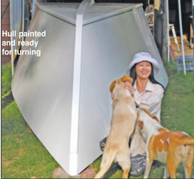
**In Part 3 we had progressed to a painted hull, almost ready to be turned over. Building a turnover frame was next, designed to create a straight-line pivot point and protect the gunwales during a rollover.**
