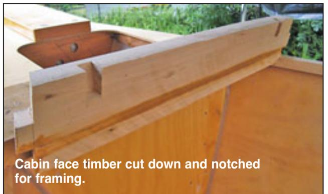
Cabin face timber cut down and notched for framing.
