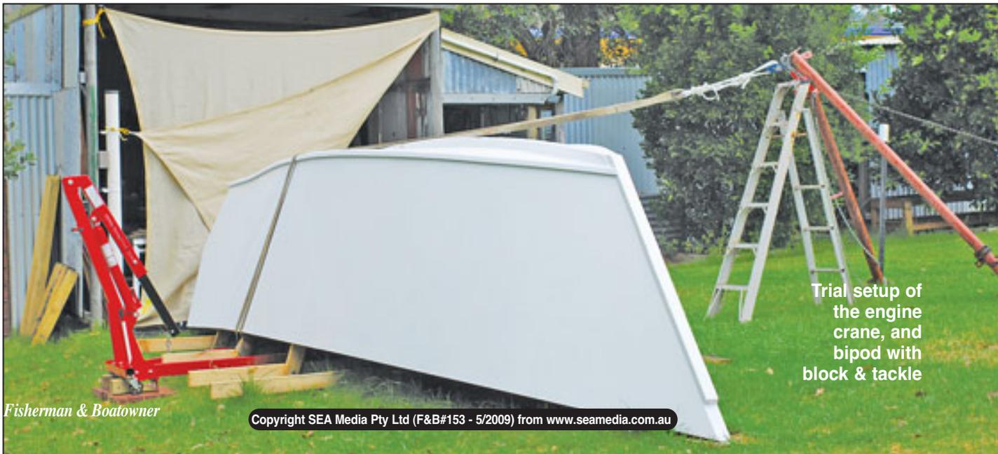
Trial setup of the engine crane, and bipod with block & tackle
