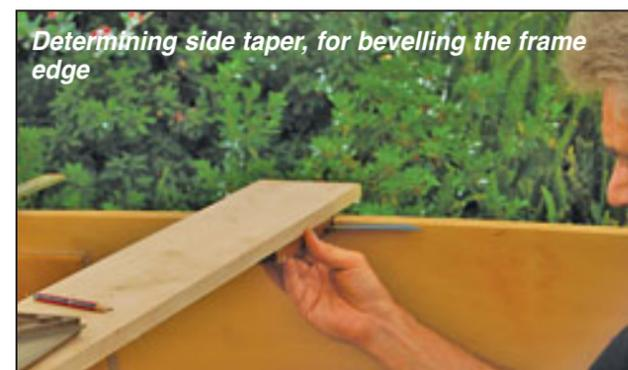
Determining side taper, for bevelling the frame edge
