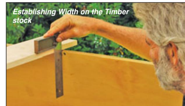
Establishing Width on the Timber stock
