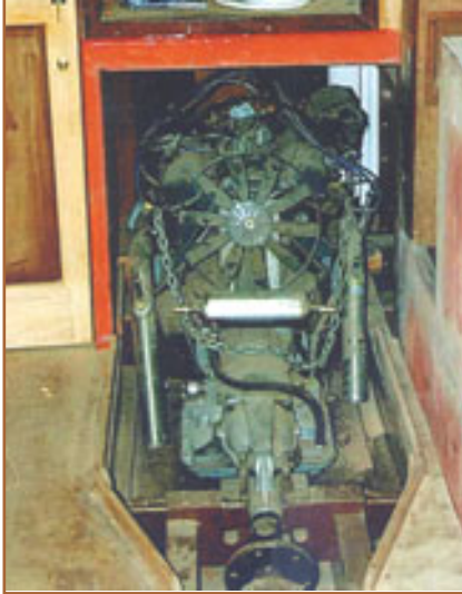
Above: The engine and transmission fitted into the boat prior to the painting being done.
