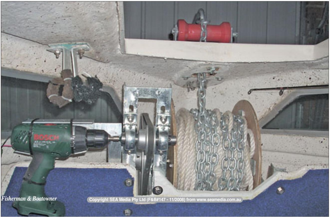
radius of about 150mm, approx 225Kg pulling power is generated. (When most of the rope is out, the pulling power is many times that).
