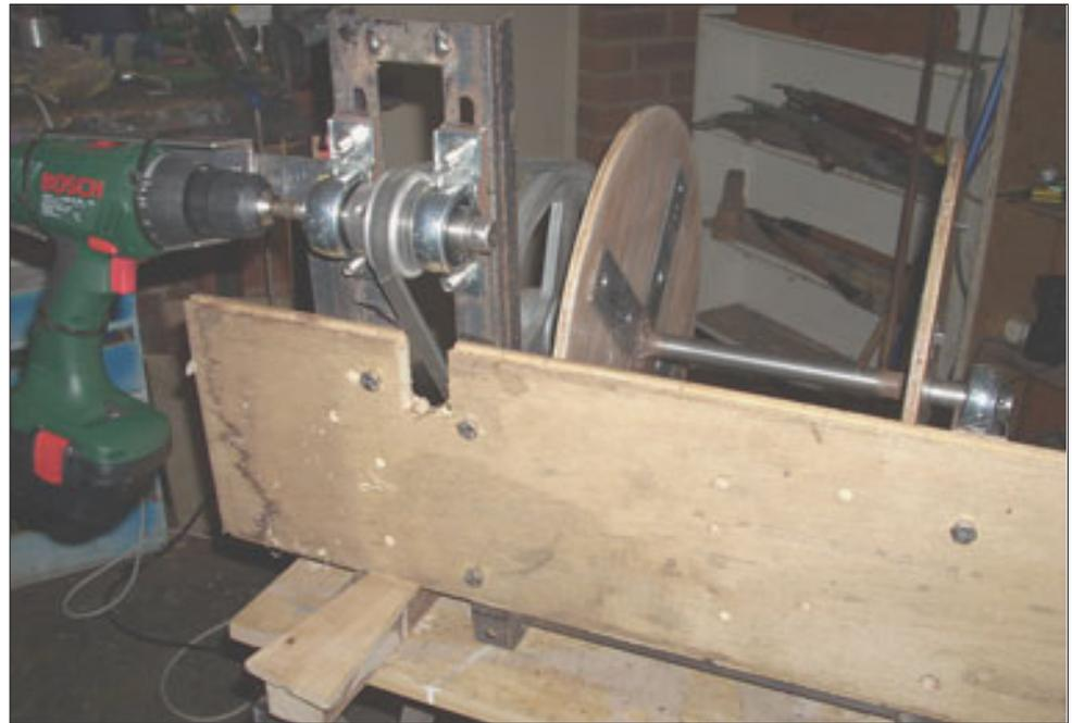
about 80rpm at the winch with the belt reduction. A belt drive was chosen because it is very cheap, keeps the drill away from wet areas and I can easily change ratios if necessary.
