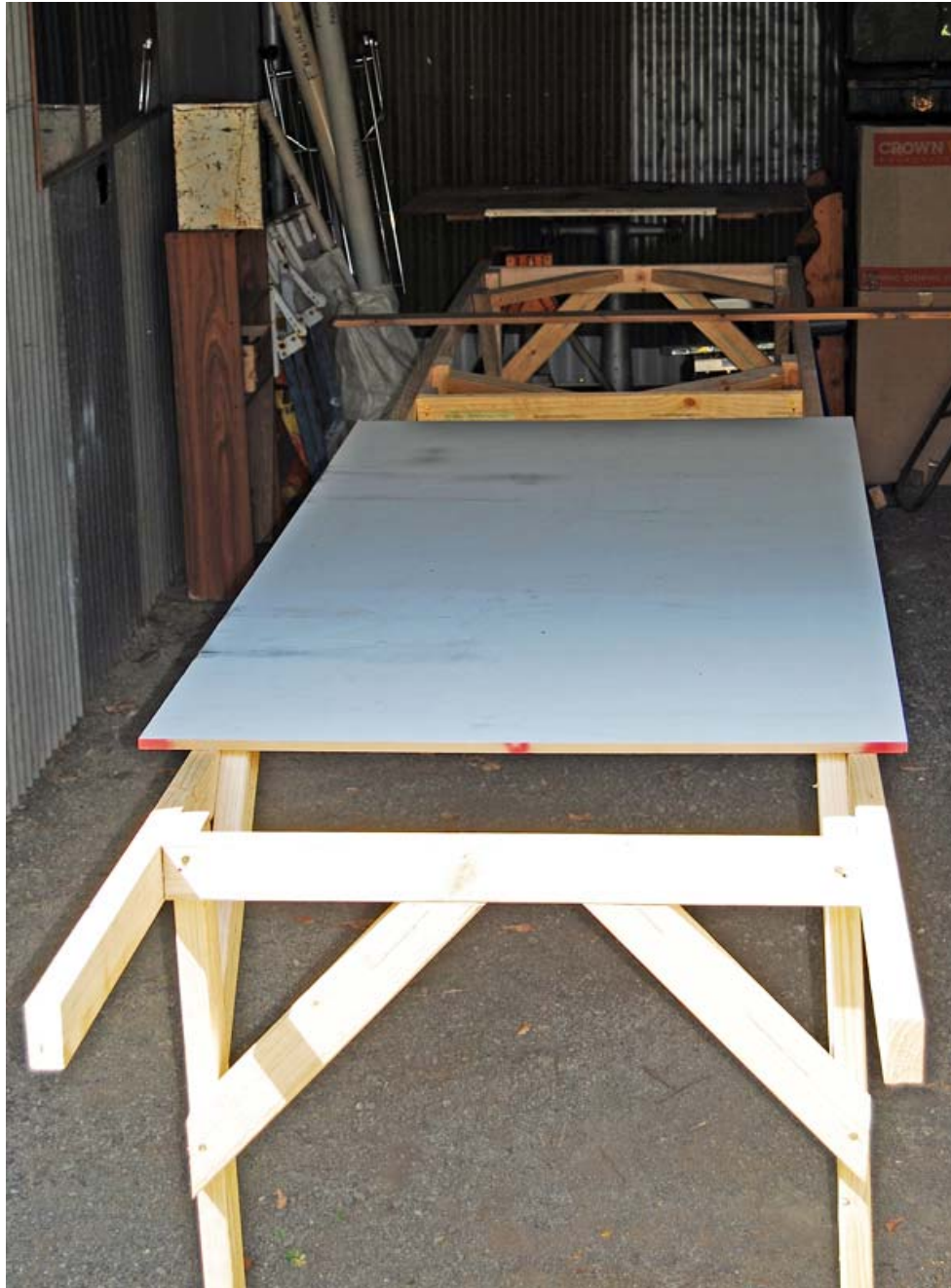
Six metre work bench, for joining ply sheets
