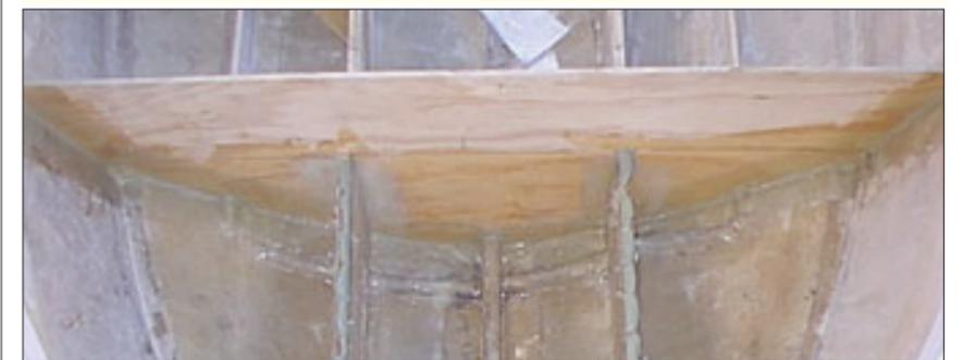
Exactly the same area as above, but seen from the front of the boat. Here, however, you can see that this forward platform also uses the forward bulkhead in the structure. While the top of the platform uses the bulkhead as a support, the bulkhead uses the platform, not in place yet, as a stiffener. Each piece adds more strength to the entire structure.
