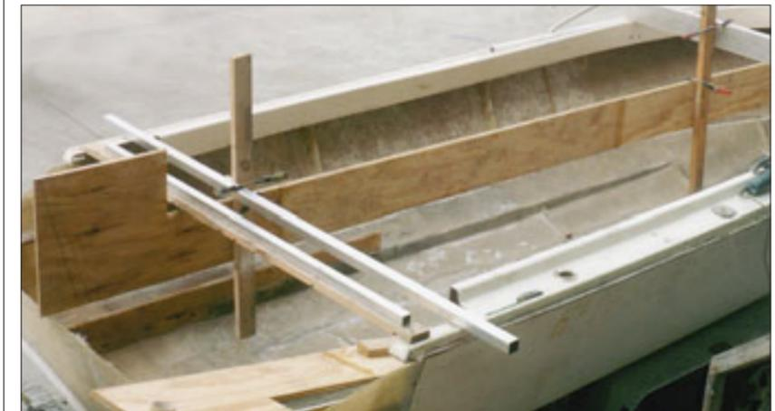
**Scribe Setup** The idea here is to get the shape of the hull where the bearer is to ultimately sit and transfer that shape to the new bearer. Then you can trim it to shape simply, with just one cut. The boat has been setup level so that the bearer can be setup level in relation to how it will actually be set into the boat.
