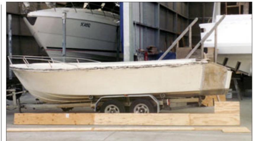
**Bearers** My two main bearers ready to be cut to the shape of the boat. They were made from 12mm ply wood double thickness and the joins were overlapped by 1.2 metres. That gave me a bearer 25mm thick. The two layers were joined with epoxy based glue to ensure that they could never separate. Epoxy glues wood better than anything and for such a critical structure is worth using. Regardless of what glue you use it must be a truly waterproof glue.
