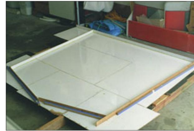
**Hardtop Mold:** My home made, one use mold for the hardtop. I was getting low on suitable material so this one looks a bit patchwork. It did, however, work out just fine. If you want the details on what is actually happening here then check out the report on DIY Fibreglassing in the library.
