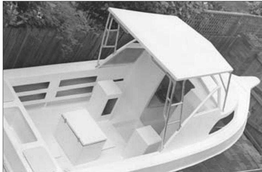
**Finished Hardtop on Boat:** The final product on the boat. The hardtop is painted in the same undercoat as the rest of the boat so this is not really final but it will show you how it will look. I'm pleased I have almost 2.0 m head room underneath the hardtop, plenty of shade and with the addition of clears it will provide a weather proof helm position. I believe the simple addition of the hardtop has made *Close Call* twice the boat she was.
