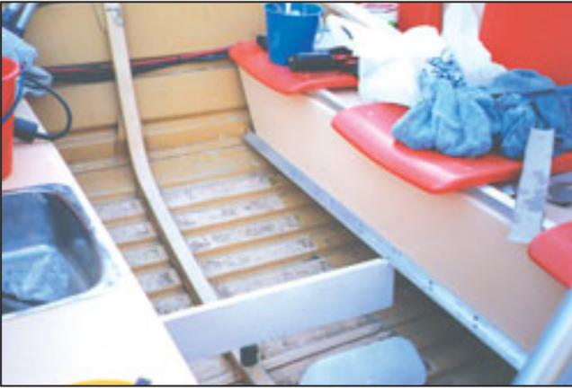
forward plywood shelf that had rotted out but still gave a good shape to trace around. If in doubt you can always cut some areas too small, just to get it to fit into the boat and then fill in up against the edge or shape by masking on some off-cut cardboard onto the main template (refer to photo).
