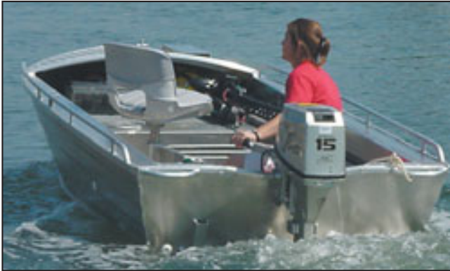
The Bluefin 3.5 is yet another fine example of how an entry level tinnie can be so easily developed into a red hot fishing platform. This boat easily fulfilled the fit-out specs listed below. Note unusual 20” transom and foam filled side decks.
