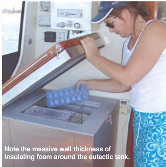
Note the massive wall thickness of insulating foam around the eutectic tank.
