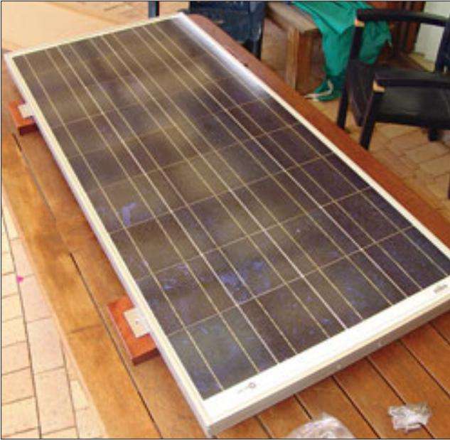
Installing the solar panels is relatively simple. The underside of the frame is pre-drilled, and because the maker's recommend that you don't install the panel (and its all-important electrical controls) hard onto the roof, we prefer to lift it up about 20-25mm so that it sits clear of the roof - and rain or hose water can then pass harmlessly underneath.
