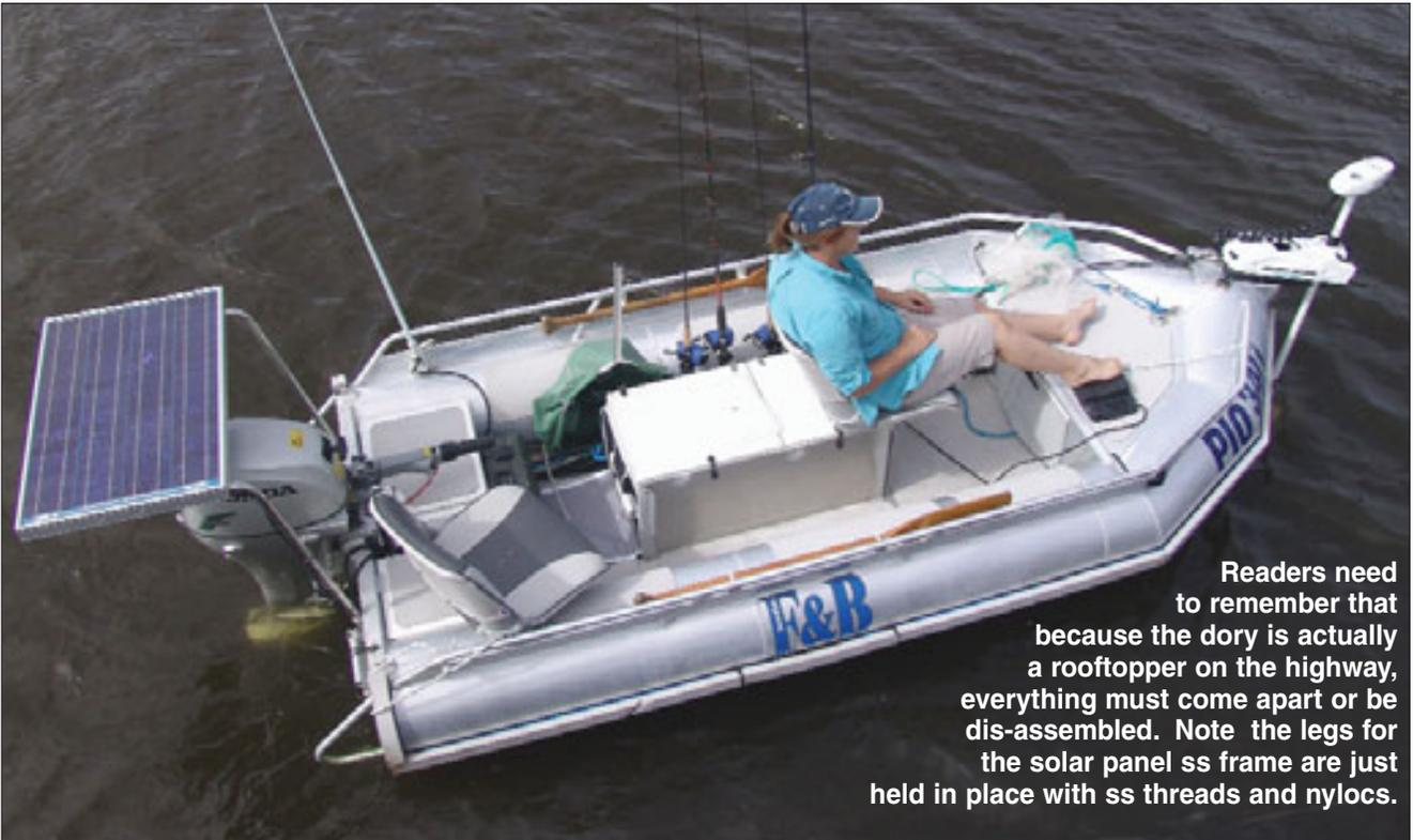
Readers need to remember that because the dory is actually a rooftoper on the highway, everything must come apart or be dis-assembled. Note the legs for the solar panel ss frame are just held in place with ss threads and nylocs.
