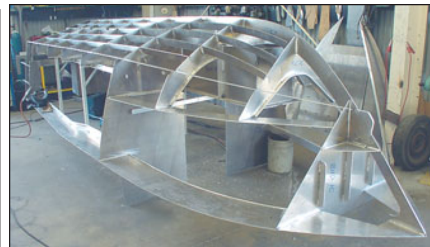
Above: Massively strong chassis matrix is accurate within 2 mm and ensures maximum hull rigidity Below: Keel section is actually solid aluminium!
