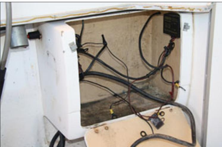
indicate the wiring technique (not!) utilized throughout this vessel – add-ons over many years by inexperienced hands, generally under dimensioned for the current expected and not inspected or maintained.
