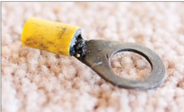
the battery box above. You will note the “open end” style, where damp and corrosion can get started, the less than professional (and certainly inadequate) crimp on the insulation which looks like it was done with pliers or a cheap, light crimper and the complete disintegration of the cable at the entry point. While the cable would have corroded from the open ring end in due course anyway, the lack of heat shrink over the cable and terminal barrel inevitably increased the rate.
