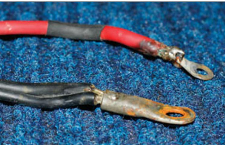
cables (windlass and main bus to the breaker panels) with a hammered "crimp" and poorly soldered into the lug (commonly known as "cocky\*\*\*\*"). Picture # 5 shows a comparison with perhaps a more suitable, albeit un-
