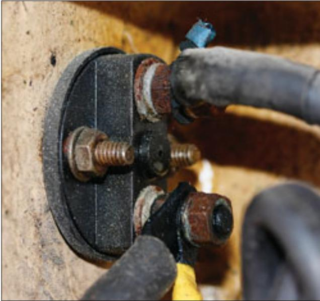
problems. Clearly it had been loose for some time, with current arcing apparent on the cable lug and washers, along with mild steel nuts which had rusted and were probably not very conductive by this stage. The isolation switch shown is an 'el cheapo", normally used in a vehicle or land based setting! With upwards of 170 amps drawn by starter motors on the engines in this vessel, there is no leeway to economize on heavy duty, waterproof switches with large terminals and stainless hardware.
