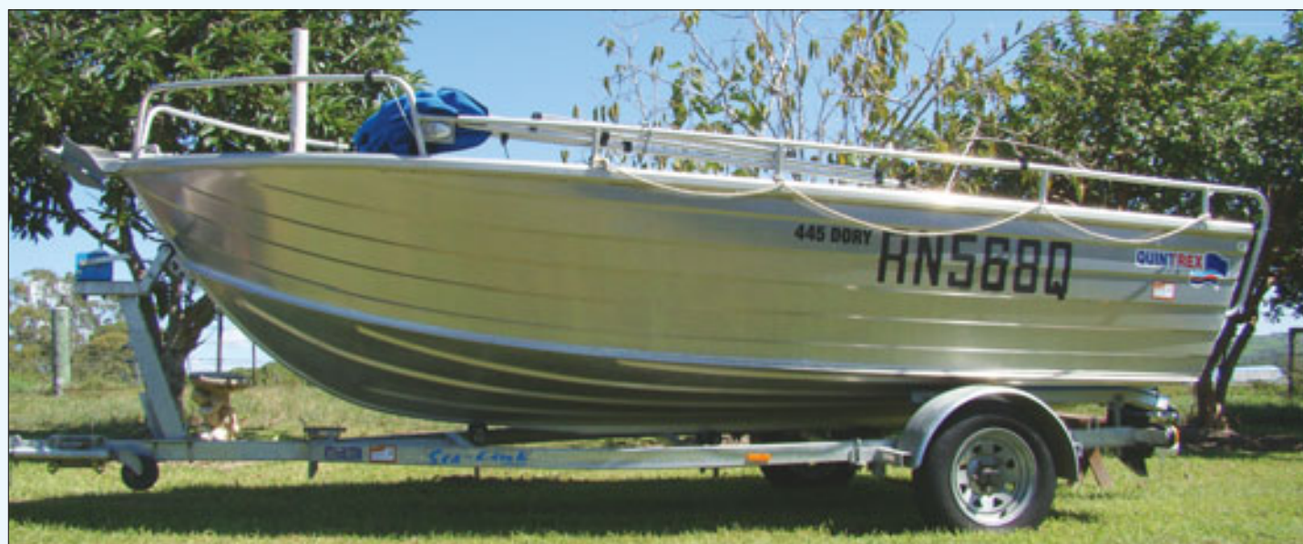
Above: Side view showing safety ropes, the bow extension, bow roller and the LED nav light mounted on the forward rail. Below: Showing the new boarding/exit step added to facilitate getting on and off at the ramp. Rail placement here is critical.
