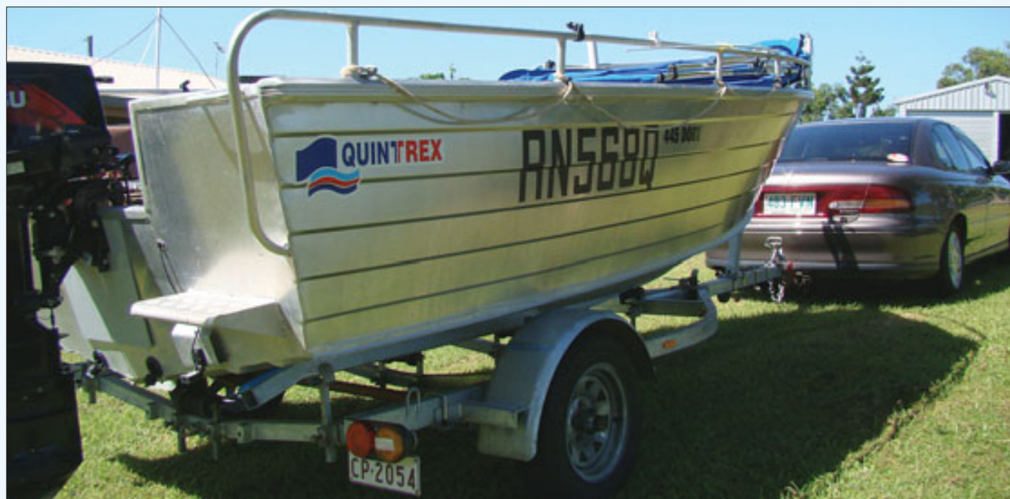
Above: Side view showing safety ropes, the bow extension, bow roller and the LED nav light mounted on the forward rail. Below: Showing the new boarding/exit step added to facilitate getting on and off at the ramp. Rail placement here is critical.
