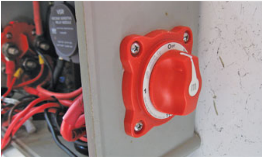
Above: Bilge pump and float switch setup Below: 4-way battery selector switch
