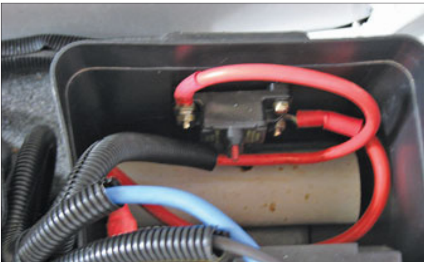
Below: Close up view of House battery and breaker
