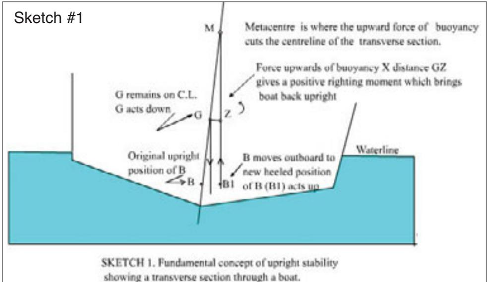
SKETCH 1. Fundamental concept of upright stability showing a transverse section through a boat.
