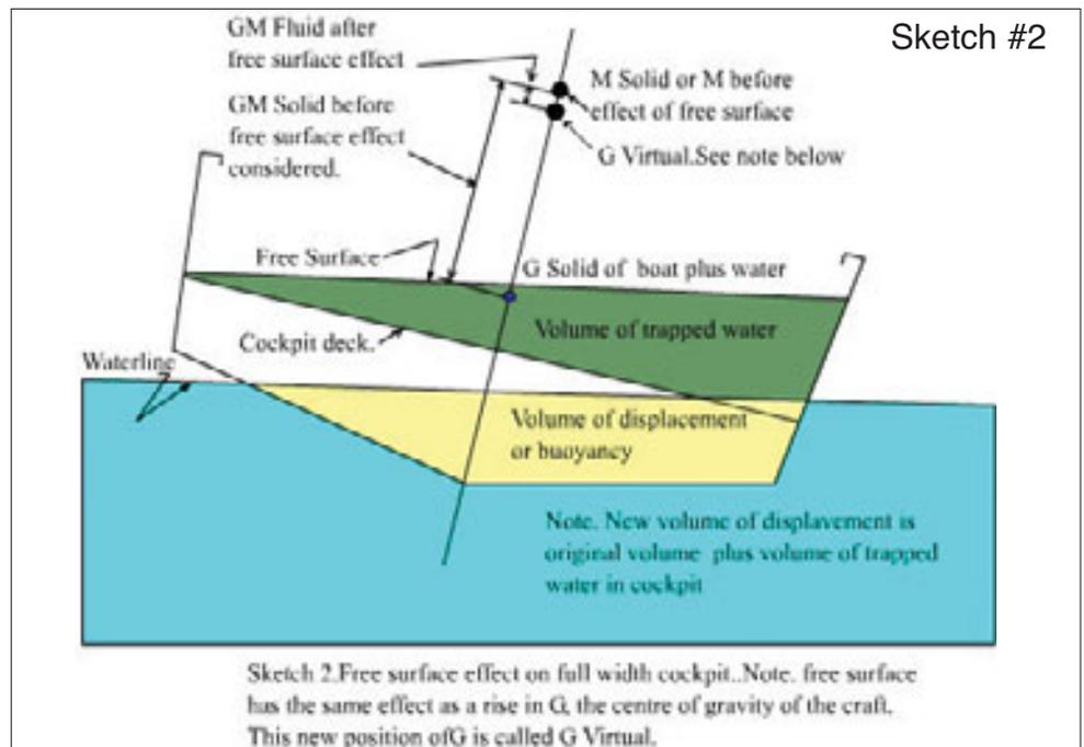
Sketch 2. Free surface effect on full width cockpit. Note. free surface has the same effect as a rise in G, the centre of gravity of the craft. This new position of G is called G Virtual.
