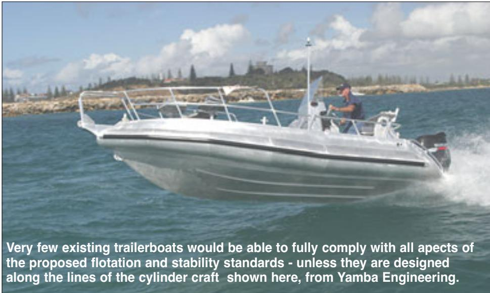
**Very few existing trailerboats would be able to fully comply with all aspects of the proposed flotation and stability standards - unless they are designed along the lines of the cylinder craft shown here, from Yamba Engineering.**
