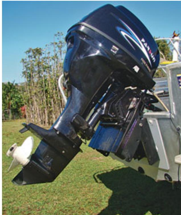
The engine is a two cylinder of approximately 500 cc which is quite big for the horsepower. It has a dummy cylinder in between the two main cylinders which acts as a dynamic balancing system to smooth out the engine, especially at idle and seems to work quite well.
