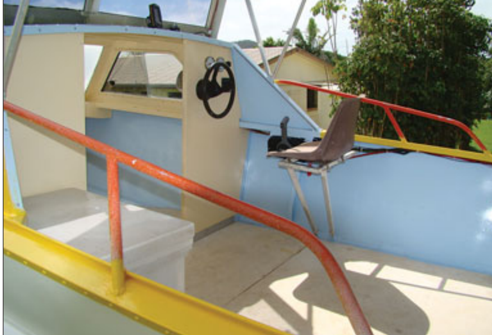
As these two pics reveal, the Trojan is now starting to load up as Neil gets into his fitting-out program. Dry hull weight has increased from about 800kg by about another 250kg.
