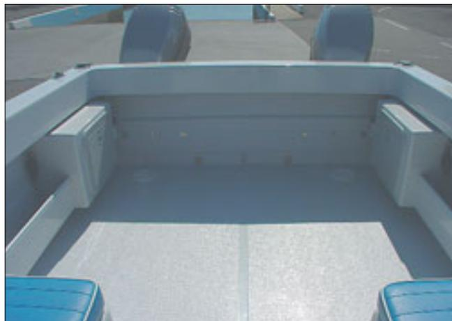
**Tight design, a good use of available space - and the preservation of a huge fishing cockpit (complete with sealed floor and a fully self draining deck) puts the Raider light years ahead of the 'tinnie brigade' of pressed mono hulls.**
