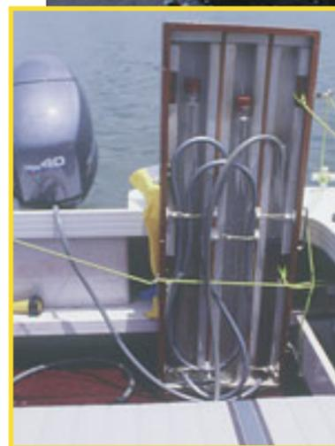
F&B's unique fuel metering system is incredibly simple but 100% accurate. It takes about 2 hours to run a full set of figures such as we have here with the Yamaha F40B.
