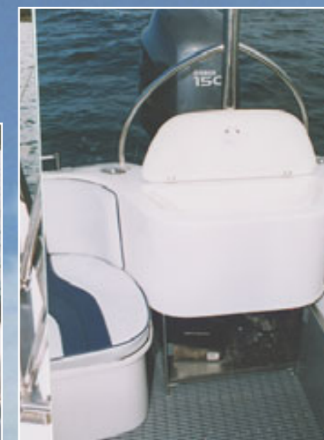
Above: Close up of the centre transom ice box/live bait tank. Note the battery box underneath.
