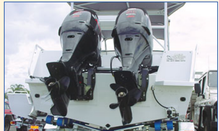
Below: This is cunning - keeping the deadrise at the transom quite moderate to boost stability and promote low speed planing. recognising that the stern will rarely if ever come clear of the water - especially with 378kg of Suzuki on the tuck.
