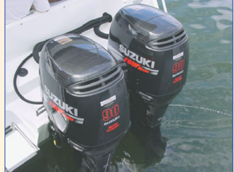
Above: A very compact duo - the latest 90hp, 4-stroke Suzukis are just about the perfect installation on this 6.4 JBS combining economy with excellent performance. Below: Isn't this a terrific layout for a spot of bottom bashing !
