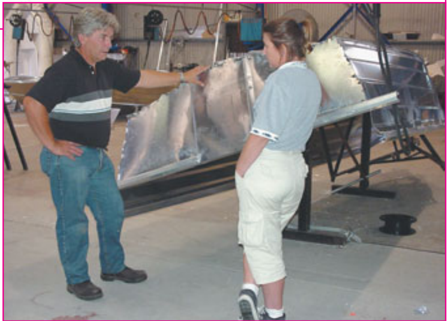
PW's original drawing of the "beachie" concept was followed very closely by the Horizon team. Below: Central to the beach-work concept was the creation of the unusual 25" transom. Here, Horizon's Bob James explains to Ruth how they achieved it working on their standard Horizon 4400 jig.
