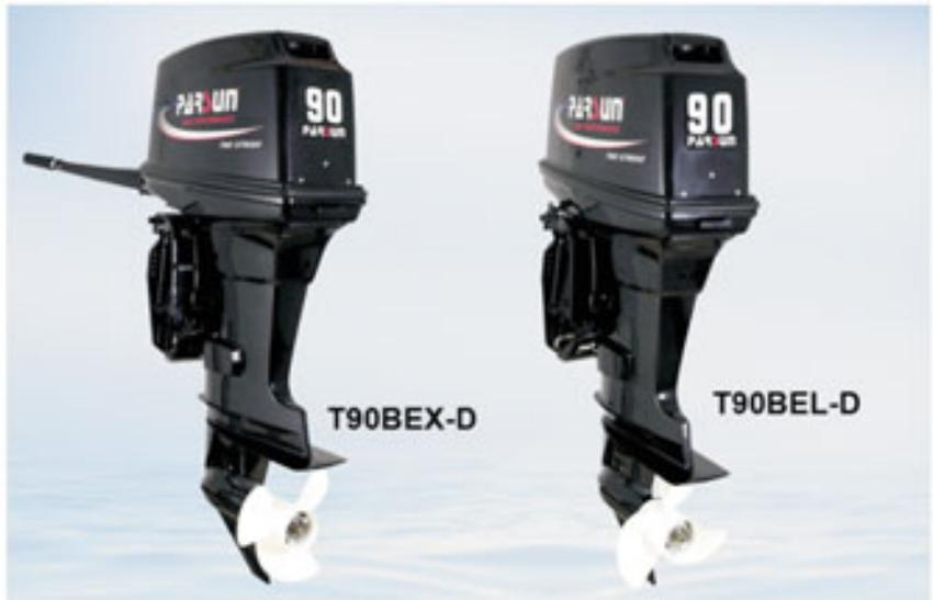
Two stroke, 3 cylinders, power trim, electric start and forward control
