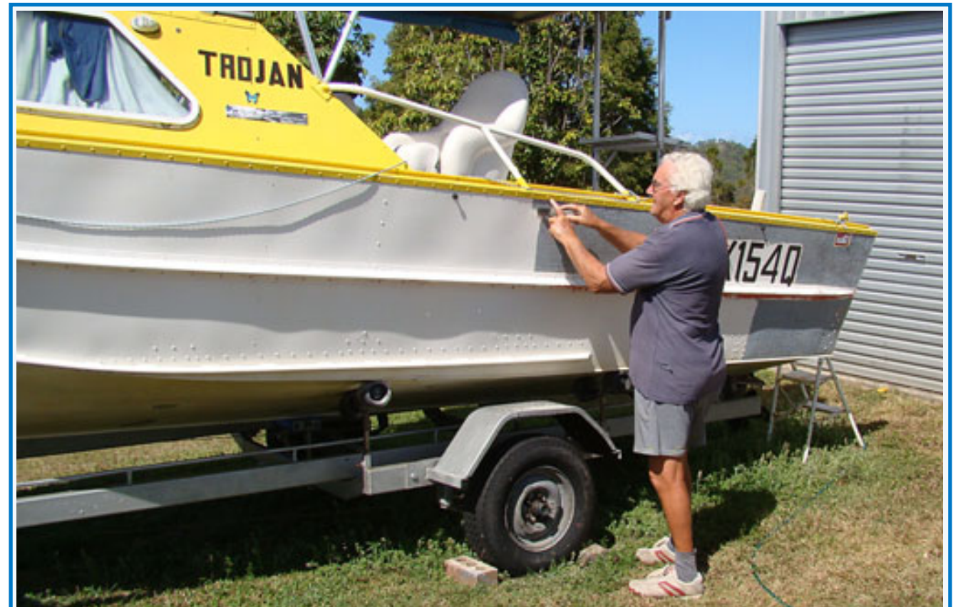
One of Neil's summer jobs ("when the wind is too strong to fish") is to refurbish the hull paint on the Trojan, a task that is surprisingly difficult for an amateur to handle - especially on a rivetted hull like this. Regular paint strippers were ineffective, sanding discs are problematic on and around the rivet heads, so paint stripper combined with an old fashioned paint scraper and lots of elbow grease proved the best - albeit painstaking - solution.
