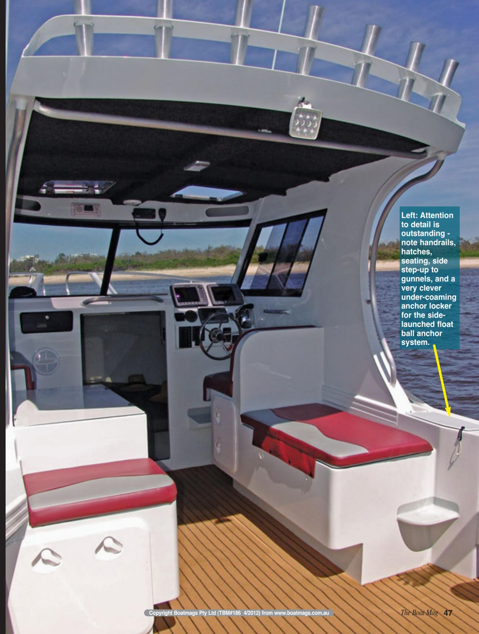
Left: Attention to detail is outstanding - note handrails, hatches, seating, side step-up to gunnels, and a very clever under-coaming anchor locker for the side-launched float ball anchor system.
