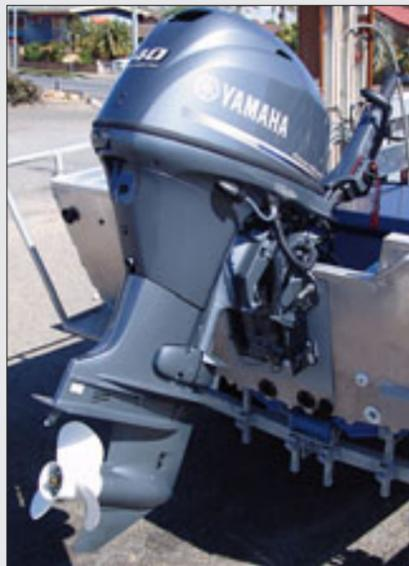
– it's all about the removal of the traditional recoil starter rope from the forward face of the engine cowling.
