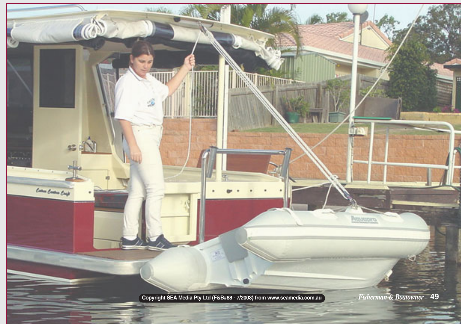
Above: " Agnes Ellen " is quite an elegant looking hull with nice proportions, accentuated by the nicely curved sheerline. Below: There's a wealth of detail to absorb here. The swimming board is critical to the design - not only does it carry the tender (raised and lowered in seconds with one hand on a simple block and tackle), it is the barbecue area, the fishing nook, swimming platform, and the walkway in and out of the boat through the excellent transom door.
