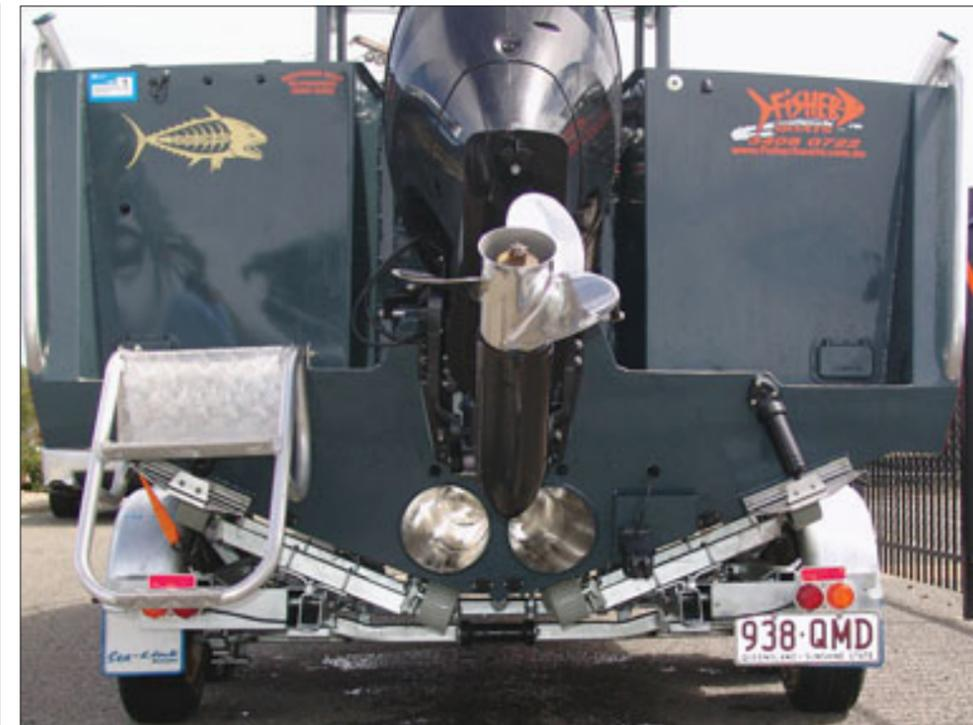
No, they are not horizontal tuna tubes (!) nor are they bits off an FA-18 exhaust. But they are part of Col Svensson's belief that if you are going to run platies with a deadrise ("Vee") as deep as this, water ballast tubes are essential for stability at rest. This is not new, just bigger than we've seen before.
