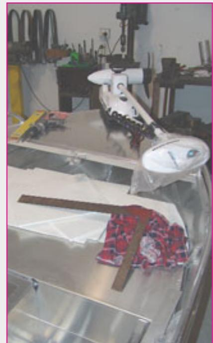
... so it is much better to bias the head to one side or the other; having it drop down and stow to a point where it will be least intrusive on the casting platform. Whether the main
