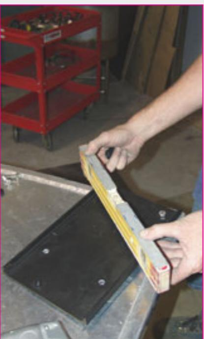
allows you to make sure the plate is nice and level - important as the Minn Kota needs to swing up and down through its operation arc nicely plumbed, so it enters the water, and runs perfectly 'square' for maximum
