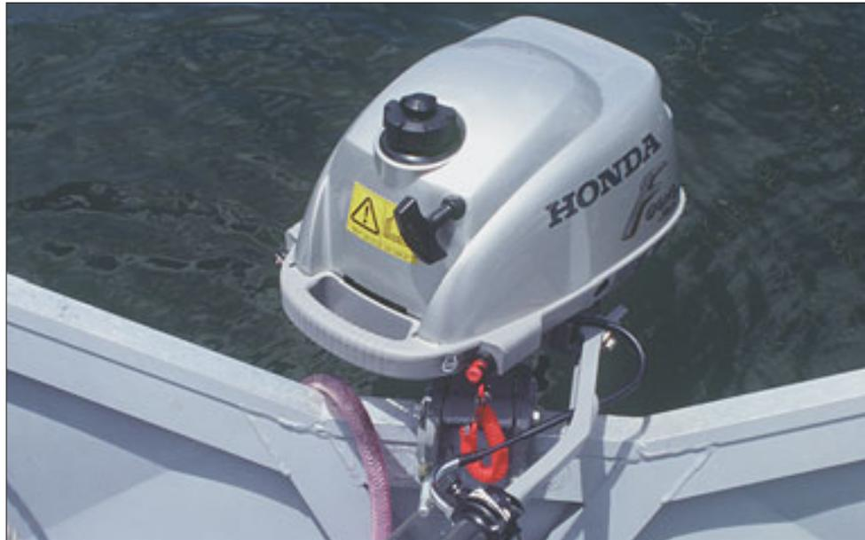
Attention to detail is excellent; simplicity the keynote. Note wide poly underbody - plastics are used extensively. It is childishly simple to use, and offers gutsy performance with quite heavy loads. Left Below: Ruth highlights the lugs it must lay on when it is stored.
