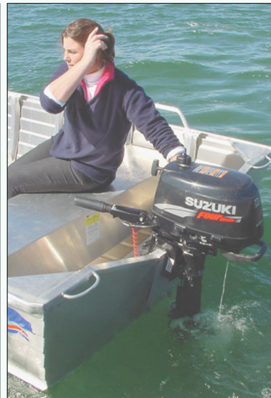
The Suzi 6hp 4-stroke outboard is a very well packaged unit, with good, man-sized handles, grab holds and gear shift lever. This model, has a rr of $1,989 which is pretty good value for a very useful 25kg 4-stroke package. By the way - apart from the inbuilt 1.5L fuel tank - you can just plug in a regular Suzi plastic tub.
