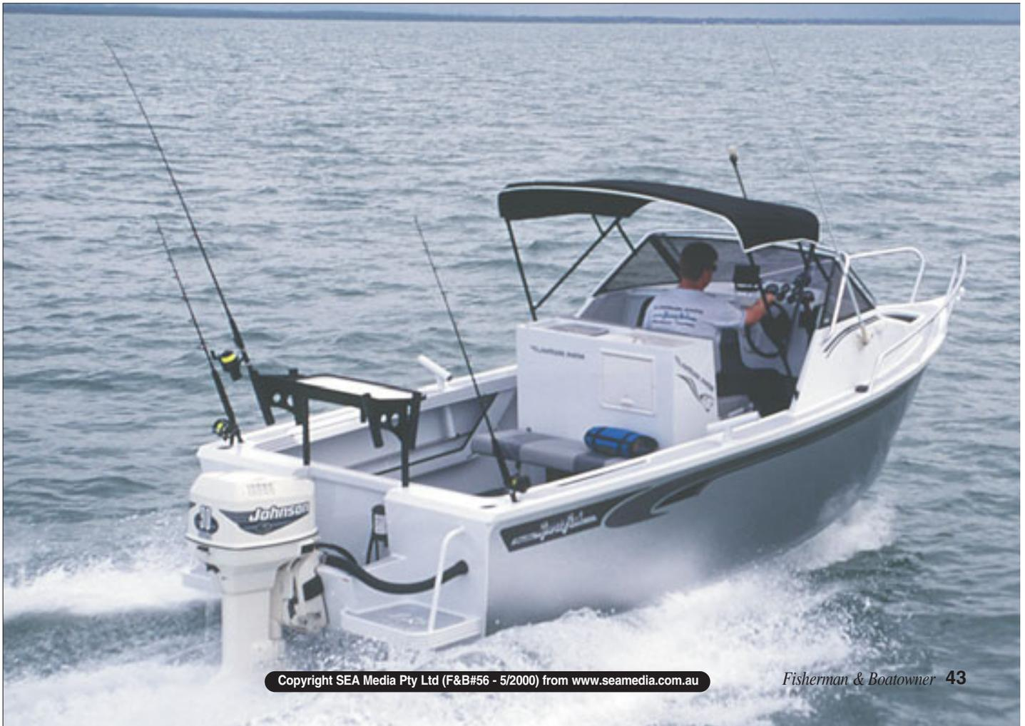
And that's what he's done. It's a very clever set-up, too. There's 1.82 m of cockpit length behind the centre work station, and combined with the boat's 2.3 m beam, created a wonderful fishing area right where it should be. He's incorporated a very space efficient transom too. So in the context of achieving maximum fishing space for his dollar, this is a really good set-up.
