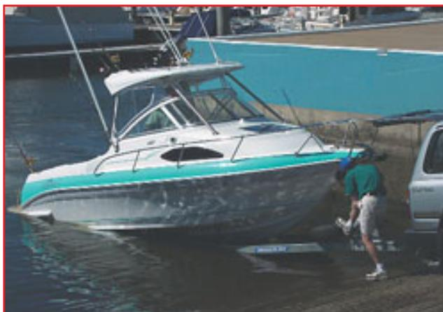
**Summary:** This is another very fine boat from the Haines Signature factory. With a towing weight of around 2.46 tonnes, it’s getting up near the upper limits of sensible towing with normal (big) 4WD’s. Having said that, on a Mackay PU 6000T trailer it’s an absolute breeze to handle on the launch ramp, and can be driven on and driven off with just one
