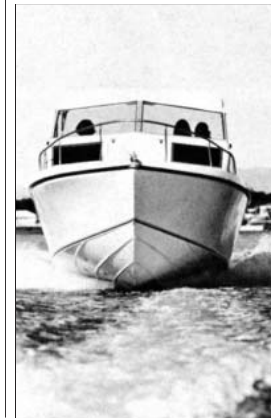
Classic illustration of a deep vee hull "working" - notice how the water is being thrown aside in "steps" from the planing strakes. Much of the hull lift is created by these strakes.
