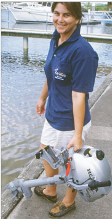
**Left:** These new little self contained 2.0 - 3.0 hp 4-stroke outboards from Honda (and Yamaha has a good one too) are amazingly good little auxiliaries – and are very useful on scanoes and inflatables. Importantly, they are light enough to man-handle out of a cupboard and back out onto a bracket - easily. They won't bring you back in from the 'Shelf, but the long shaft models will definitely get (and keep) you and your family out of trouble - until professional help arrives.
