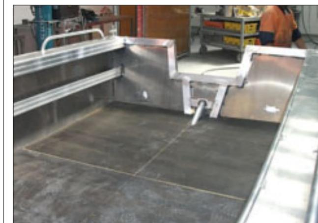
Looking forward we can also test fit the ply deck panels to the casting deck. Again these panels will be covered in carpet before being screwed or riveted in place after fitting the foam. We recommend painting the ply with a clear coat for extra protection before applying the carpet. The carpet may be glued over the ply, or screwed along the edges, or held in with Velcro. We have decided to
